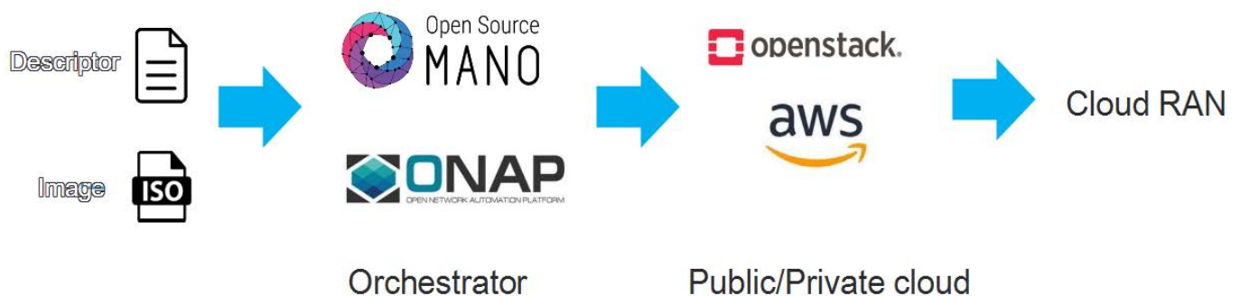
Figure 7 Cloud RAN Deployment details
